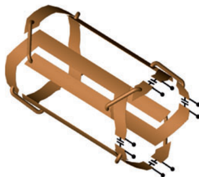
Figure 22. Four-loop volume coil fabricated from foil saddle coil elements with wire jumpers spanning the crossover points.
