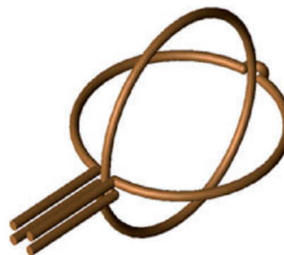
Figure 14. Crossed wire loops depicted as a two-coil orthogonal pair. The B_1 field is in the plane perpendicular to the four-feed terminals.
