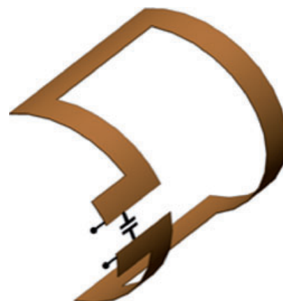
Figure 8. Rectangular, sample-conforming saddle-shaped, foil solenoid surface coil. The B_1 field in this case is detected primarily horizontal in this diagram.
