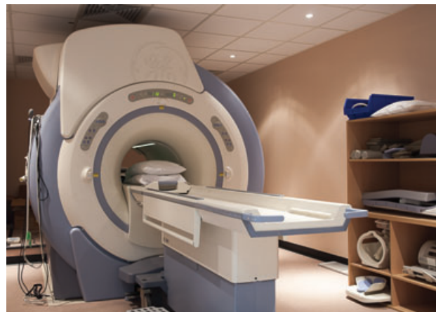
Figure 2. Clinical MRI magnet. The controls on the front panel allow landmarking of a region of interest (ROI) on the patient and control of the position of the motorized bed. The shelves to the right store RF coils when not in use
